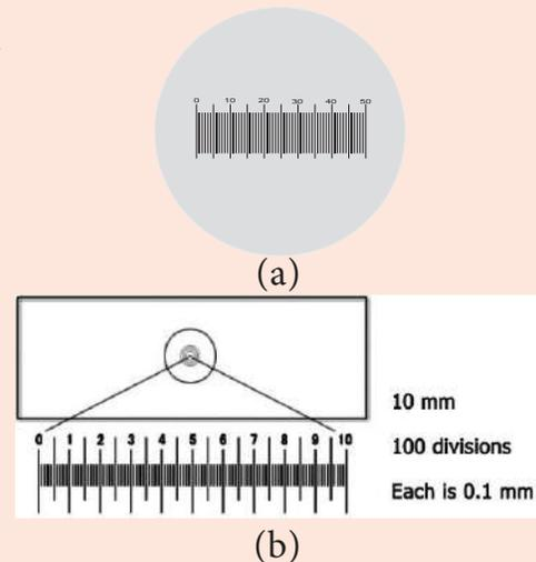
**Figure 6.5:** a. Ocular micrometre; b. Stage micrometre
