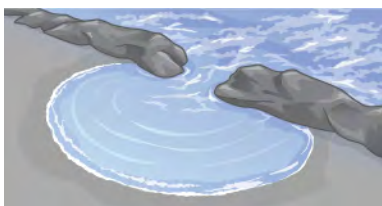
Figure 17.6 Ocean waves pass through an opening in a reef, resulting in a diffraction pattern. Diffraction occurs because the opening is similar in width to the wavelength of the waves.
