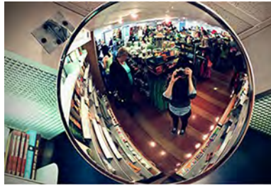
Figure 16.11 Security mirrors are convex, producing a smaller, upright image. Because the image is smaller, a larger area is imaged compared with what would be observed for a flat mirror; hence, security is improved. (credit: Laura D'Alessandro, Flickr)
