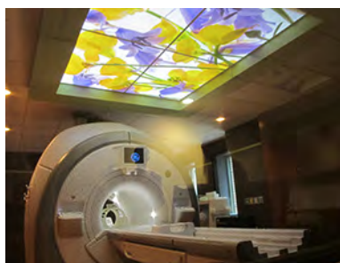
Figure 20.12 Instrument for magnetic resonance imaging (MRI). The device uses a cylindrical-coil electromagnet to produce for the main magnetic field. The patient goes into the tunnel on the gurney. (credit: Bill McChesney, Flickr)
