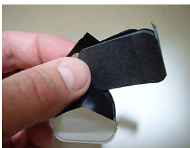
Figure 22.22 Film badges contain film similar to that used in this dental X-ray film. It is sandwiched between various absorbers to determine the penetrating ability of the radiation as well as the amount. Film badges are worn to determine radiation exposure. (credit: Werneuchen, Wikimedia Commons)
