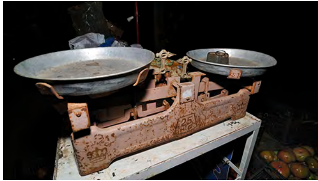
Figure 1.19 A double-pan mechanical balance is used to compare different masses. Usually an object with unknown mass is placed in one pan and objects of known mass are placed in the other pan. When the bar that connects the two pans is horizontal, then the masses in both pans are equal. The known masses are typically metal cylinders of standard mass such as 1 gram, 10 grams, and 100 grams. (Serge Melki)
