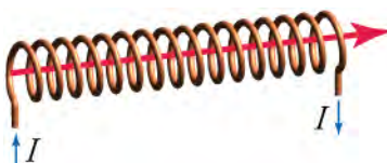
Figure 20.14 A wire coil with current running through as shown produces a magnetic field in the direction of the red arrow.
