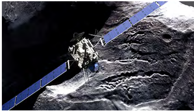
Figure 1.10 The Rosetta spacecraft, with its large and revolutionary solar panels, carried the Philae lander to a comet. The lander then detached and landed on the comet's surface. (European Space Agency)
