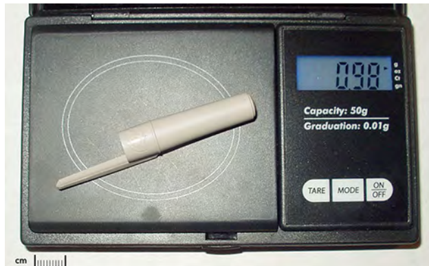
Figure 1.20 Whereas a mechanical balance may only read the mass of an object to the nearest tenth of a gram, some digital scales can measure the mass of an object up to the nearest thousandth of a gram. As in other measuring devices, the precision of a scale is limited to the last measured figures. This is the hundredths place in the scale pictured here. (Splarka, Wikimedia Commons)
