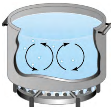
Figure 11.6 Convection plays an important role in heat transfer inside this pot of water. Once conducted to the inside fluid, heat transfer to other parts of the pot is mostly by convection. The hotter water expands, decreases in density, and rises to transfer heat to other regions of the water, while colder water sinks to the bottom. This process repeats as long as there is water in the pot.
